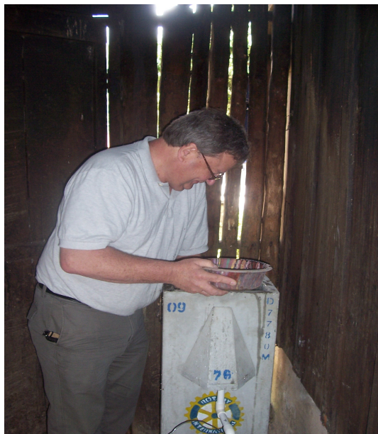
Robin Baron of Freeport loading sand into filter photo by Rick Rhea
